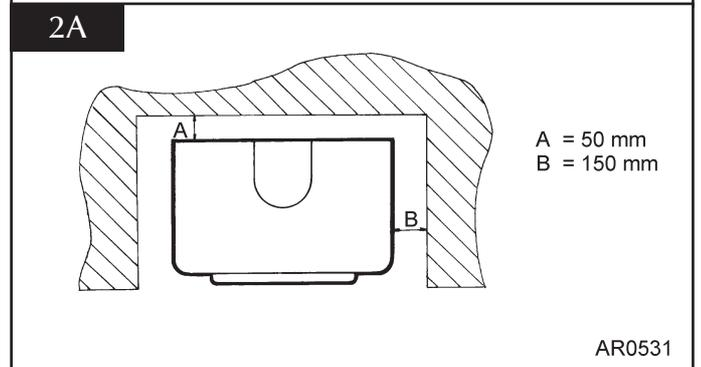
In a non-combustible recess attention must be given to allowing adequate clearance at the sides and rear of the stove, so that a spillage test can be performed, and the controls reached.
