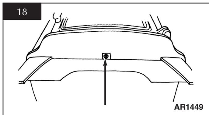
10.2 Undo the M5 nyloc nut from the bottom of the burner unit and remove the aeration plate. See diagram 19.
