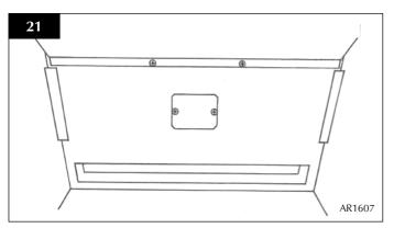
9.4 Disconnect the two slender wires. Undo the two taptite screws and remove the sensor and the two plastic spacers. See diagram 22.
