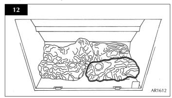
5.4 Place log D across from the rear log A to log B on the lefthand side. There are cut-outs in both logs for location. See diagram 13.
