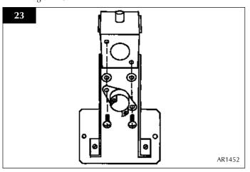
9.6 Feed the cable back through the hole as you replace the bracket. When the bracket is located correctly it will sit flush with the back panel without force required. If not positioned correctly the bracket will sit at an angle. See Diagram 24.
