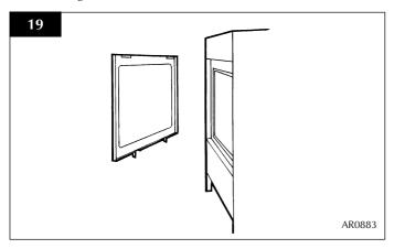
NEVER OPERATE THE STOVE WHEN THE DOOR IS REMOVED OR WHEN THE GLASS IS BROKEN.
