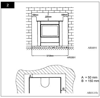
NOTE: IN A NON-COMBUSTIBLE RECESS ATTENTION MUST BE GIVEN TO ALLOWING ADEQUATE CLEARANCE AT THE SIDES AND REAR OF THE STOVE, SO THAT A SPILLAGE TEST CAN BE PERFORMED AND THE CONTROLS REACHED.
