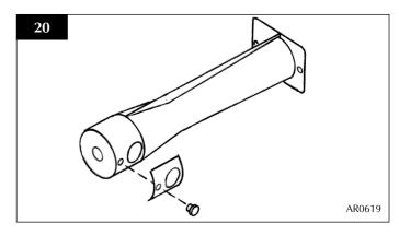
10.5 Reassemble in reverse order with correct aeration plate(s).NOTE: Even if no aeration plate is required, the small screw(s) must be replaced.
