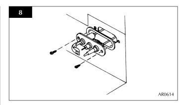
3.5 To remove the pilot injector, undo the compression nut on the pilot feed pipe and withdraw the injector which will be hooked onto the olive. When replacing an injector always make sure it is hooked onto the olive before inserting it into
