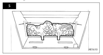
7.2 Place log B on the left-hand side of the burner with the location bar on the underside of the log fully located in the long slot of the burner. Make sure the log is as far to the left as possible. See diagram 6.
