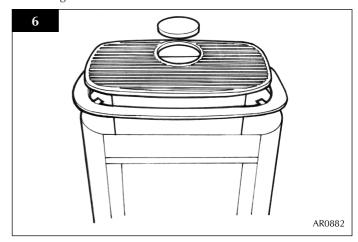
3.10 Check the pull of the flue system by applying a lighted smoke pellet to the flue system opening. If there is a definite flow into the chimney, proceed with the installation. If not, warm the chimney for a few minutes.
