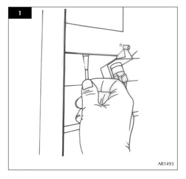
1.2 If there are any extractor fans in adjacent rooms, the test must be repeated with the fans running on maximum and interconnecting doors open.
