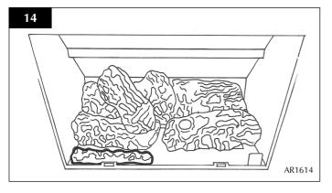
5.6 Place the second ash panel to the right of the first, with the pointed end of the panel fitting into the V shape. This panel should locate on the screw holes of the burner skin. Ensure that both logs are horizontal to the burner ports.
