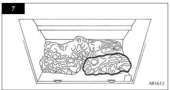
7.4 Place log D across from the rear log A to log B on the left-hand side. There are cut-outs in both logs for location. See diagram 8.
