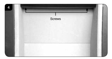
4.3 The baffle can now be removed through the front of the appliance.
