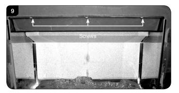
5.5 The baffle can now be removed through the front of the appliance.
