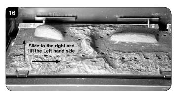
6.5 Slide the burner back to the left and out of its location. IMPORTANT: Take care when removing the burner not to damage the ceramic pad with the pilot unit attached.
