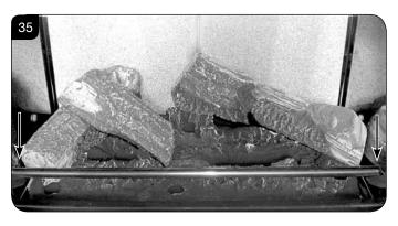
8.20 Place Log A across Log C. There is a hole on the underside of Log A which fits over the raised stud on Log C to secure in place. The small cut out on the left side of the log rests onto the log guard, see Diagram 36.
