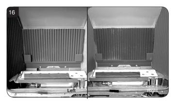
5.10 Locate the top panel on top of the sides and rear by lifting it up and forward inside the box.
