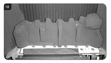
5.13 Place the front coal centrally in the channel at the front of the tray. The relationship between the front coal and the flame baffle is shown, see Diagram 19.
