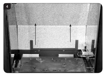
4.5 Slide the lower rear liner up and out of the lower bracket, see Diagram 5.
