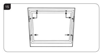
8.2 Replace ALL of the securing screws ensuring that a screw is present in all fixing slots.
