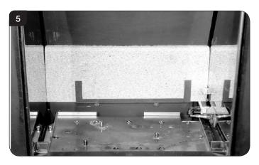
4.6 Replace all parts in reverse order ensuring the cutouts in the rear of the lower panel fit over the screws on the back of the firebox, see Diagram 6.
