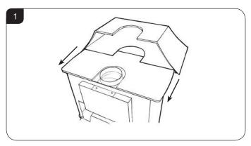
3.5 Make sure the appliance top fits into the guide along the bottom of the canopy, see Diagram 2.
