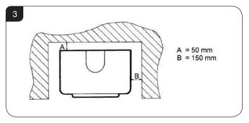
5.5 The above dimensions provide adequate clearance to combustible materials. It may be necessary to add additional clearance so that spillage tests can be performed when necessary.
