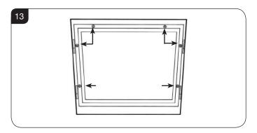
7.11 Replace ALL of the securing screws ensuring that a screw is present in all fixing slots.
