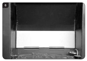
4.7 With the liners and baffle removed the firebox is clear for cleaning and maintenance, see Diagram 7.
