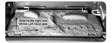
5.4 Slide the burner back to the left and out of its location. **IMPORTANT: Take care when removing the burner not to** damage the ceramic pad with the pilot unit attached.
