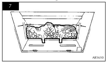
Place log B on the left-hand side of the burner with the location bar on its underside slid into the long slot of the burner • Make sure the log is as far left as possible, Diagram 8
