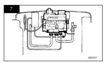
NOTE: TAKECARENOTTODISCONNECTTHESENSORWIRES FOR THE GAZCO FLUE SURE SYSTEM WHEN YOU REPLACE THE THERMOCOUPLE TO THE BACK OF THE GAS VALVE.
