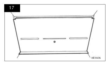
9.3 • Undo the two screws at the back of the firebox and carefully withdraw the bracket
