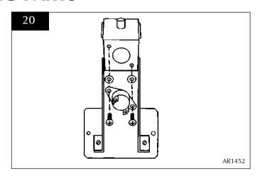
9.6 • Feed the cable back through the hole as you replace the bracket. When the bracket is located correctly it sits flush with the back panel with no force. If not positioned correctly the bracket sits at an angle, Diagram 21.
