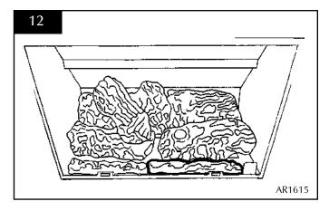
Place log E across from the rear of log A to log C on the right-hand side using the shaped cut-outs as location guides. The front of the log should sit on the front ash panels and should fit tight to log C, Diagram 13
