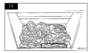
Place log E across from the rear of log A to log C on the right-hand side using the shaped cut-outs as location guides.
