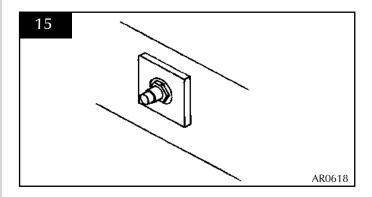
**•** Holding the injector with a spanner to undo the feed pipe
