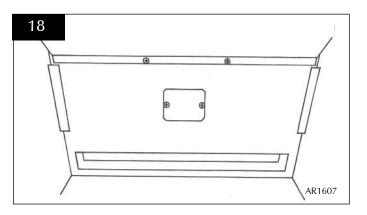
9.4 Disconnect the two slender wires. Undo the two taptite screws and remove the sensor and the two plastic spacers. See Diagram 19.
