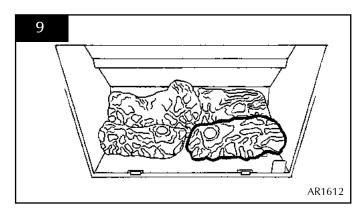
Place log D across from the rear log A to log B on the left-hand side. There are cut-outs in both logs for location, Diagram 10
