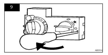
Disconnect the other end of the ignition lead from the valve body
