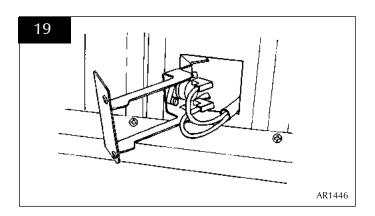
Refit the new sensor, ensuring that the plastic spacers are between the sensor and the bracket. Refit the leads. See Diagram 20
