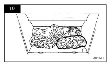
Place log D across from the rear log A to log B on the left-hand side. There are cut-outs in both logs for location. See Diagram 11
