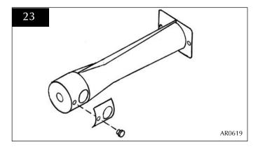
10.2 • Reassemble in reverse order with correct aeration plate(s).
