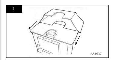
• Make sure the canopy fits into the guide along the bottom of the canopy, Diagram 2
