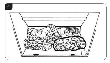
7.4 Place log D across from the rear log A to log B on the lefthand side. There are cut-outs in both logs for location, see Diagram 10.
