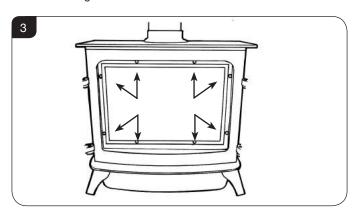
3.2 Lower the frame down to clear the top edge before lifting clear, see Diagram 4.
