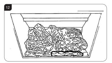
7.7 Place log E across from the rear of log A to log C on the right-hand side using the shaped cut-outs as location guides. The front of the log should sit on the front ash panels and should fit tight to log C, see Diagram 13.
