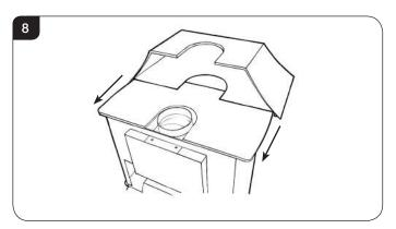
4.2 Make sure the appliance top fits into the guide along the bottom of the canopy, see Diagram 9.
