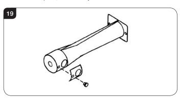
11.5 Reassemble in reverse order with correct aeration plate(s). Note: Even if no aeration plate is required, the small screw(s) must be replaced.
