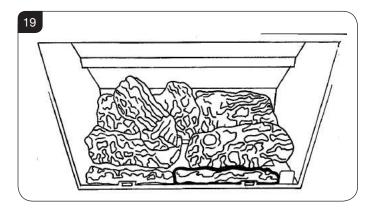
8.8 Place log E across from the rear of log A to log C on the right-hand side using the shaped cut-outs as location guides. The front of the log should sit on the front ash panels and should fit tight to log C, see Diagram 20.
