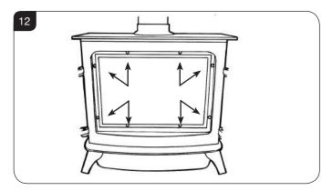
6.6 Lower the frame down to clear the top edge before lifting clear, see Diagram 13.
