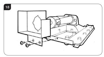
11.4 Refer to the technical specification and databadge to check the gas type and its required aeration plate. Change the aeration plate, if necessary.
