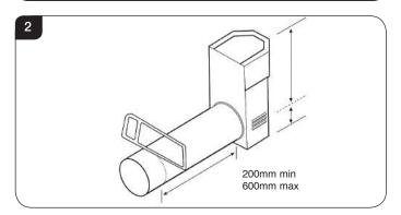
Terminal dimensions: 395 x 200 x 200 mm (H x W x D) Guard supplied Cut to length as required on site, see Diagram 2.
