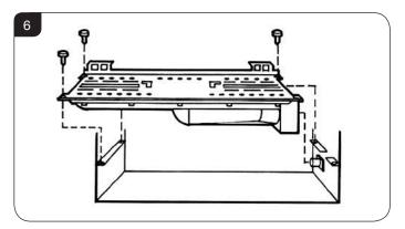
4.6 To replace the burner, engage the venturi over the injector ensuring the burner sits on top of the fixing bracket. Push the burner to the right and whilst holding, insert the three fixing screws.
