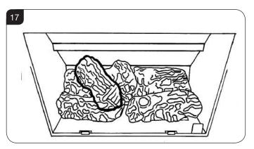
8.6 There are two ash panels which lay across the front of the burner. Place the panel with the flat edge facing the left side of the firebox. There are location holes on this log which fit over the screw holes on the burner.
