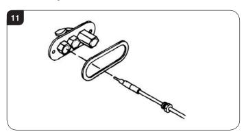
5.10 Undo the thermocouple from the back of the gas valve, see Diagram 12.
