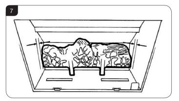
7.2 Place log B on the left-hand side of the burner with the location bar on its underside slid into the long slot of the burner. Make sure the log is as far left as possible, see Diagram 8.
