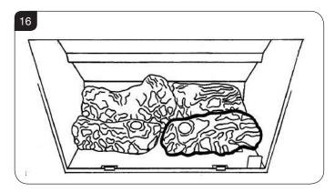
8.5 Place log D across from the rear log A to log B on the lefthand side. There are cut-outs in both logs for location, see Diagram 17.
