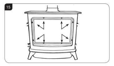
7.10 Replace ALL of the securing screws ensuring that a screw is present in all fixing slots.
