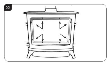
9.3 Replace ALL of the securing screws ensuring that a screw is present in all fixing slots.
