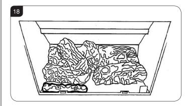
8.7 Place the second ash panel to the right of the first, with the pointed end of the panel fitting the V shape and fitting the screw holes on the burner. Ensure that both logs are horizontal to the burner ports.
