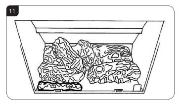
7.6 Place the second ash panel to the right of the first, with the pointed end of the panel fitting the V shape and fitting the screw holes on the burner. Ensure that both logs are horizontal to the burner ports.
