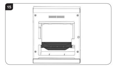
6.5 Fit the plug supplied into the hole where the riddling mechanism is normally located and secure with bolt and clamp (also supplied), see Diagram 16.
