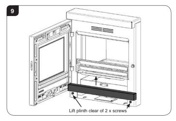
8.3 If the plinth is too loose it can be adjusted via the 2 x side screws and half lock nuts behind it. The plinth is designed to sit tight but still be removable.
