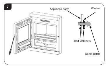
7.3 Once the desired setting has been achieved ensure the lock nuts are tightened against the appliance body.
