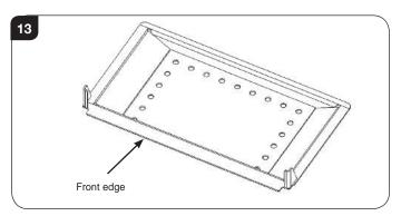
6.1 Remove the riddling mechanism from the appliance (see Pre-Installation, Section 6).
