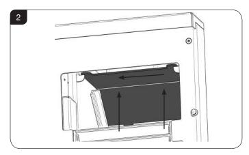
5.4 In one movement lower the other side of the baffle and move it sideways to clear its supports on both sides of the appliance. Pull the baffle toward you and out through the door opening.
