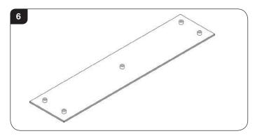
2.4 Place the glass top, feet down, on the appliance. Ensure the glass top is flush with the front and sides of the steel top.
