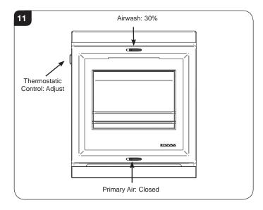
5.20 Close the Primary Air Controls and adjust the Airwash Control to approximately 30% open. 5.21 Control the temperature and hot water output using the Thermostatic Control.
