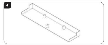
2.2 With the door open, fix the steel top in position from the underside using the 2 x M8 x 20 hex head screws and 2 x M8 crinkle washers.
