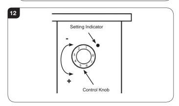
5.23 The exact setting of the thermostat and the Manual Air Controls may need slight adjustment by trial and error to suit requirements.
