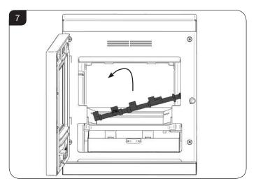
6.9 Lift the multi-fuel frame and rotate to remove from the firebox.
