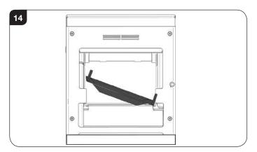
6.4 Place tray flat on the fixings on the firebed, see Diagram 15.
