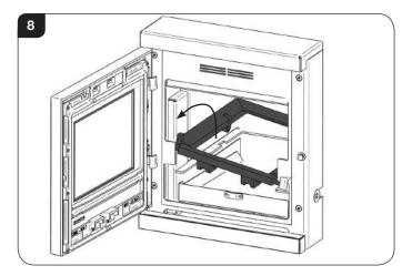
6.10 Replace the internal components in reverse order.
