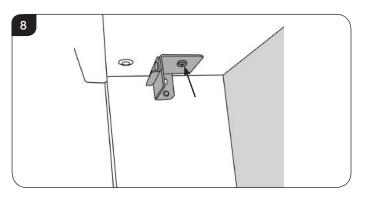
5.5 Carefully pull the side brackets down at an angle and pull forward to remove, see Diagram 9. Note: Each bracket will only fit on one side.
