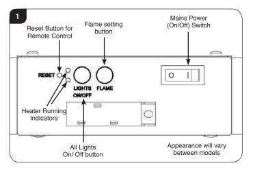
Note: The appliance will lose the memory for the light functions when the switch is set to the Off Position or the remote runs out of power.
