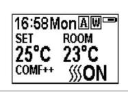
If the heater is on in the current period, pressing the button will turn the heater off.
