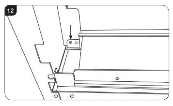
6.2 The bracket and the fuel bed can now be lifted out of the appliance, see Diagram 13.
