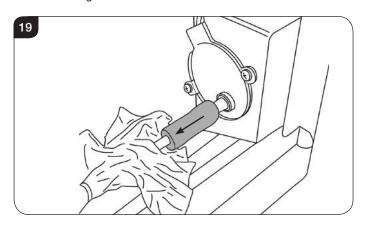
8.5 Gently withdraw the spindle from the support brackets at an angle, see Diagram 20.
