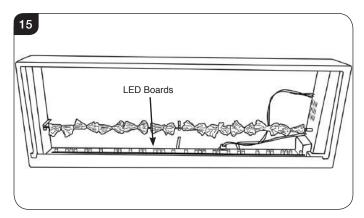
7.3 The LED boards are coupled together at the end of each board and held in place by clips, see Diagram 16.
