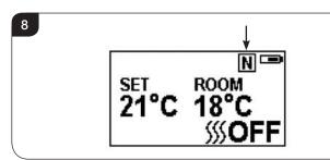
2b.22 Press the '+' or '-' button to adjust the setting temperature from 17 °C to 25°C.
