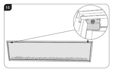
3.7 Supporting the glass, loosen and remove the 2 clamps. These can be unscrewed using just finger tips. 3.8 Carefully tip the glass forward and lift out of the lower tray to remove from the appliance, see Diagram 16. The clamp can be used to aid removal.
