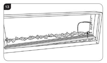
6.3 Replace in reverse order. NOTE: The flexible fuel bed locates in a groove in the bracket, see Diagram 14.
