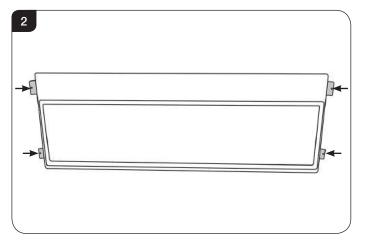
3.4 The fireplace can now be positioned in the opening. Level the appliance, and attach the unit to the frame using the fixing holes provided, see Diagram 3.
