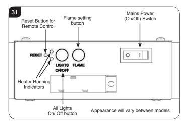
Resetting of the remote control is necessary if the appliance operates wrongly due to external interference signal and the remote control is not in use.
