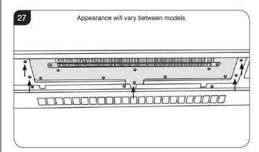
11.4 Carefully lower the Heater Assembly. This will require a slight tipping motion to clear the edge, see Diagram 28. NOTE: The Heater Assembly has wires attached.
