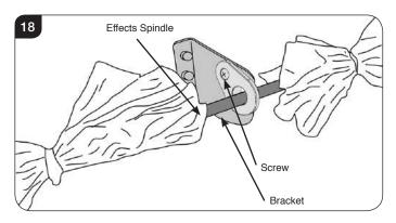
8.4 The Effects Spindle is attached to the Effects Motor by a rubber sleeve.
