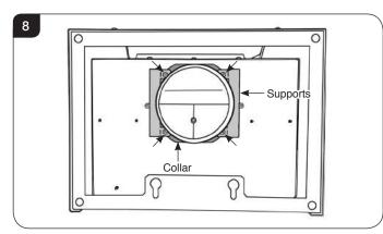
4.5 Swap the flue spigot **only** with the Blanking Plate on the rear of the appliance, see Diagram 9.
