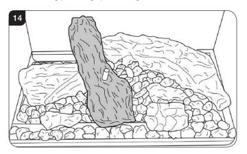
7.7 The fourth log fits onto the locating pin and rests on the second log, see Diagram 15.
