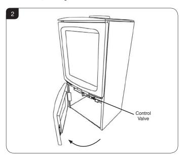
The valve has two controls, see Diagram 3.
