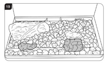
8.5 The second log is positioned on the right hand locating pin, and rests against the back liner, see Diagram 20.
