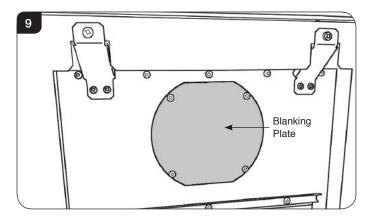
4.6 Attach the decorative flue blanking plate support bracket to the underside of the cast top using the screws provided. Ensure the folded return is pressed against the cast top, see Diagram 10.
