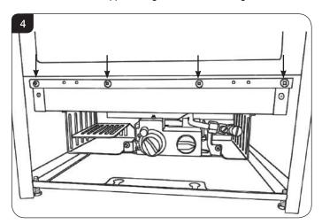
3.2 The frame can be removed by lifting the hooks clear of the slots from the bottom of the frame and lifting away from the appliance, see Diagram 5.
