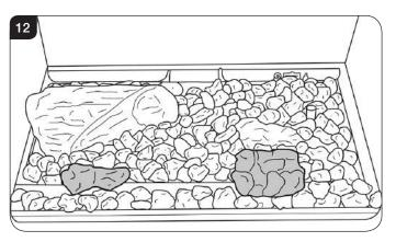
7.5 The second log is positioned on the right hand locating pin, and rests against the back liner, see Diagram 13.
