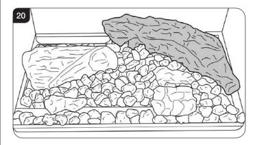
8.6 The third log rests on the first and second logs with the locating pin facing up, see Diagram 21.
