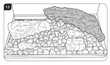
7.6 The third log rests on the first and second logs with the locating pin facing up, see Diagram 14.
