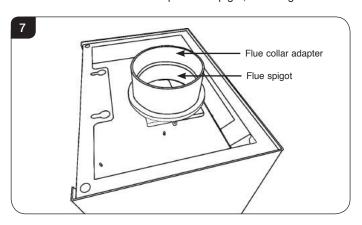
4.4 Remove the flue collar adapter supports and the flue spigot by removing the 4 screws, see Diagram 8.
