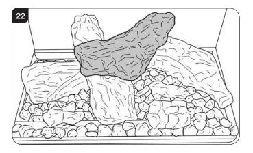
8.8 Spread a liberal amount of the Embaglow fibres provided on the sections highlighted, see Diagram 23.
