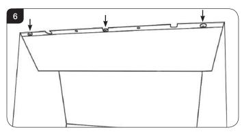
4.2 The baffle can now be removed through the front of the appliance.
