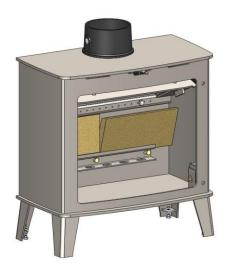
Pull the top edge of the Rear Brick forward and lift the brick out of the Stove.
