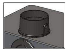
Secure in place using the M6 nuts and washers. Slide the remaining gasket on to the studs of the flue collar or blanking plate and secure in place on the back plate. Unless the optional flue damper is being fitted, blank off the damper handle holes in the flue collar using the two M8 coach bolts.
