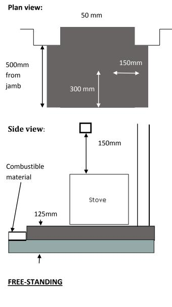
If the stove is not to stand in an appliance recess, it may stand wholly above a hearth made of noncombustible board / sheet material or tiles, at least 12mm thick.
