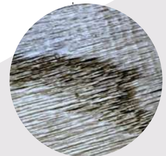
Excessive corrosion on cooking plate
