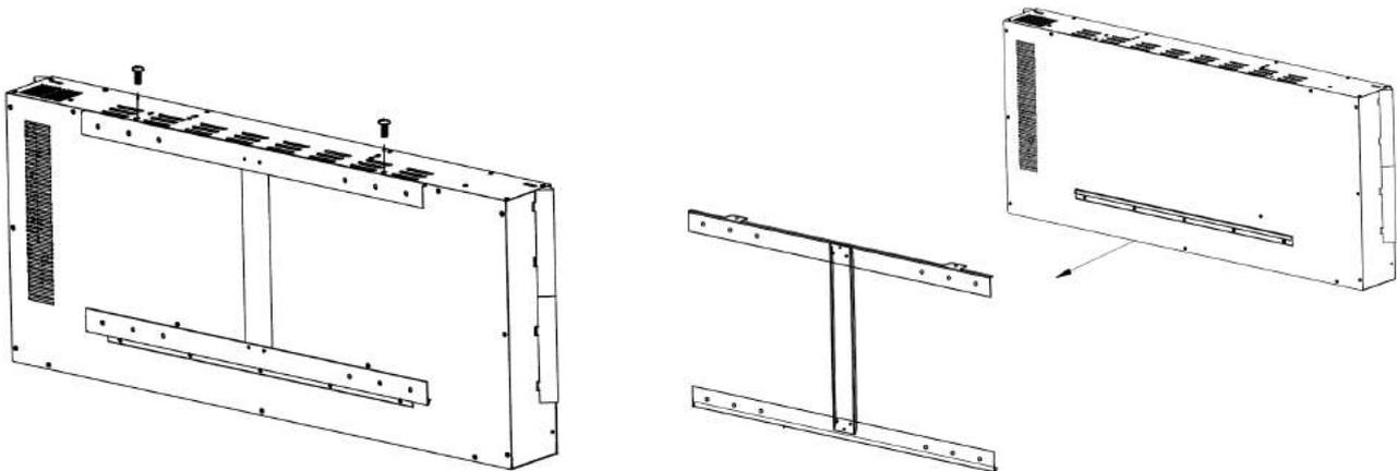
Step 2: Choose a solid and plain wall. Position the mounting bracket where the appliance is to be installed on the wall and ensure that the bracket is level. Using a pen mark the 4 holes through the 4 holes on the mounting bracket as shown below (Figure 2)
