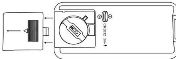
3. The battery has two sides, one with a button feature, and the other is flat.
