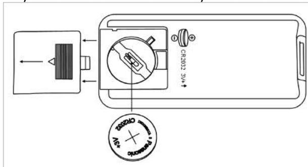
4. Insert the battery with the button side into the remote control, and make sure the battery is firmly seated into the remote control.
