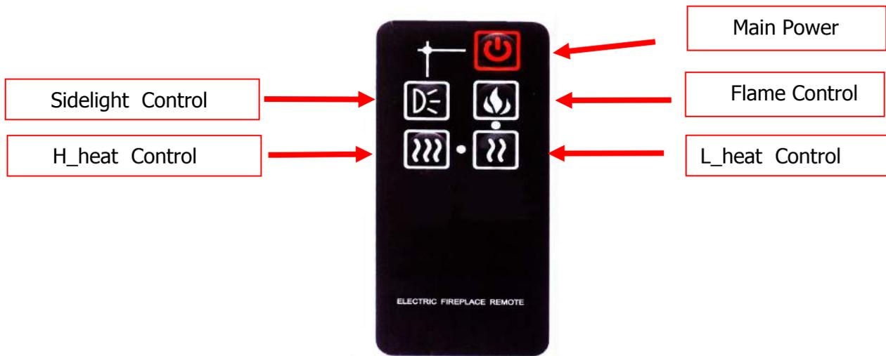
These remote control buttons work exactly the same as the buttons on the front panel of the fireplace/heater. See the FIREPLACE/HEATER section above to review the side plate panel button functions, and familiarize yourself with the remote control.
