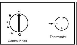
bed) should light. If it does not, repeat the operation a few times to purge any air in the pipe. Continue to hold knob for 15 - 20 second to establish the pilot and then release. If pilot fails to establish, turn off, wait 1 minute then repeat lighting procedure. Rotate the red knob to high flame to light then back to the desired flame position. If no gas comes through rotate the black knob (thermostat) to a hotter room setting and the fire will light.
