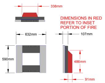
Hearths - For hearth mounting (or if the fire is less than 200mm above the ground) then the hearth must protrude at least 100mm in front of the fire and 50mm to either side. A minimum hearth of 732mm wide x 207mm deep is required, the hearth must be a minimum of 12mm thick and be of a non combustible material. The surface on which the appliance is to stand must be flat, level and square to the back panel. Failure to observe this could result in the appliance leaning away from the fireplace.
