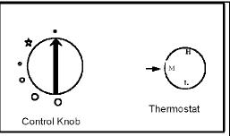
should light. If it does not, repeat the operation a few times to purge any air in the pipe. Continue to hold knob for 15 - 20 second to establish the pilot and then release. If pilot fails to establish, turn off, wait 1 minute then repeat lighting procedure. Rotate the red knob to high flame to light then back to the desired flame position. If no gas comes through rotate the black knob (thermostat) to a hotter room setting and the fire will light.
