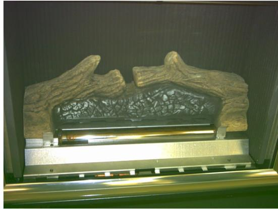
8.1.1 Carefully place the rear (largest) log piece on the support platform behind the burner. Ensure the base of the log piece is flat on the support and that the rear is pushed back as far as possible. Ensure that no part of this log piece is in contact with the tubular burner (Fig.8).
