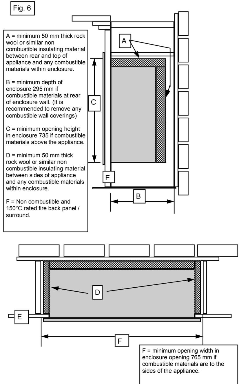
7.1.4 A suitable non combustible support platform shall be constructed within the enclosure for the appliance to sit upon.
