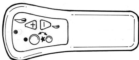
10.2.1 Batteries – The handset takes a standard 9v battery. This should be changed annually to ensure the fire continues to operate correctly. It can be accessed through a flap on the back of the handset.
