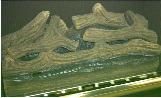
8.1.4 Place the remaining log to the right hand side of the fuel bed to bridge the front and rear log pieces. The stubby branch should nestle down and be located in the notch on the right of the rear log piece. The other end of the log shall come to rest on the branch stub protruding from
