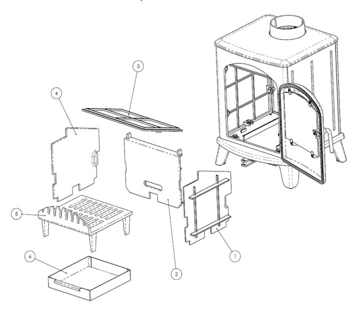
To refit the internals follow the numbered sequence from 1-6. The firebricks should fit quite snug however small gaps are acceptable due to cast iron tolerances. Be careful not to trap or squash fingers at this stage.
