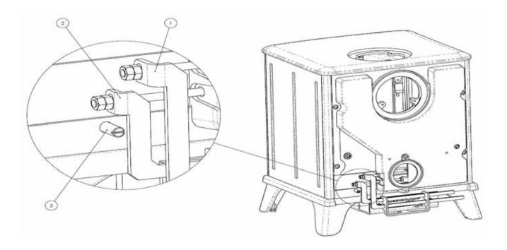
If the stove is being installed into a property which is not in a smoke control zone, you can simply screw the threaded rod into the stove (this will allow the slider to fully close and cut off the air supply)
