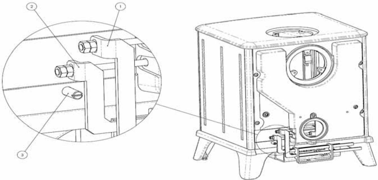
If the stove is being installed into a property which is not in a smoke control zone, you can simply screw the threaded rod into the stove (this will allow the slider to fully close and cut off the air supply)
