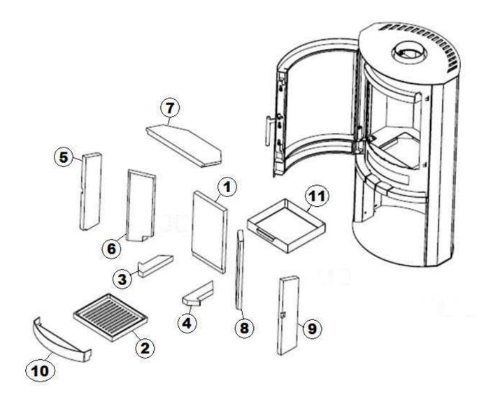
To install these parts follow the numbered sequence above, to un-install simply follow the sequence in reverese.
