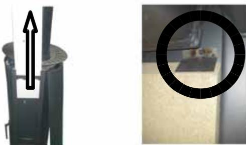
4. Slide the fibre-board up and out of the stove, you should now be able to see one final nut. With the nut removed you should be able to remove the retaining clip that is holding the internal side firebrick.
