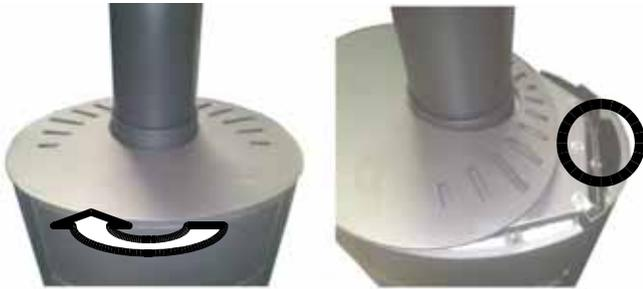
1. Lift and rotate the lid to one side to reveal the top fixings for the side panels, slacken and repeat for both sides. 10mm spanner required.
