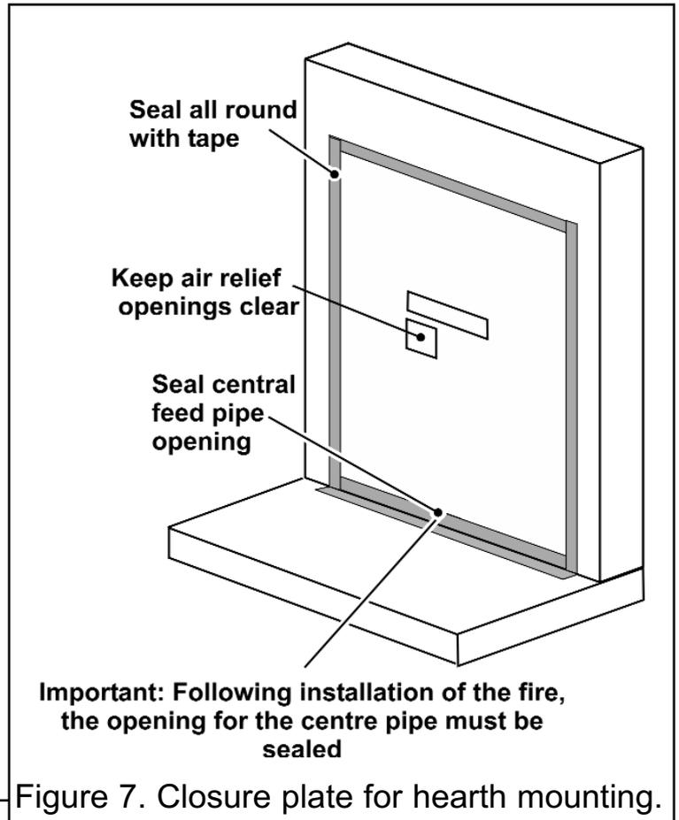
Figure 7. Closure plate for hearth mounting.
