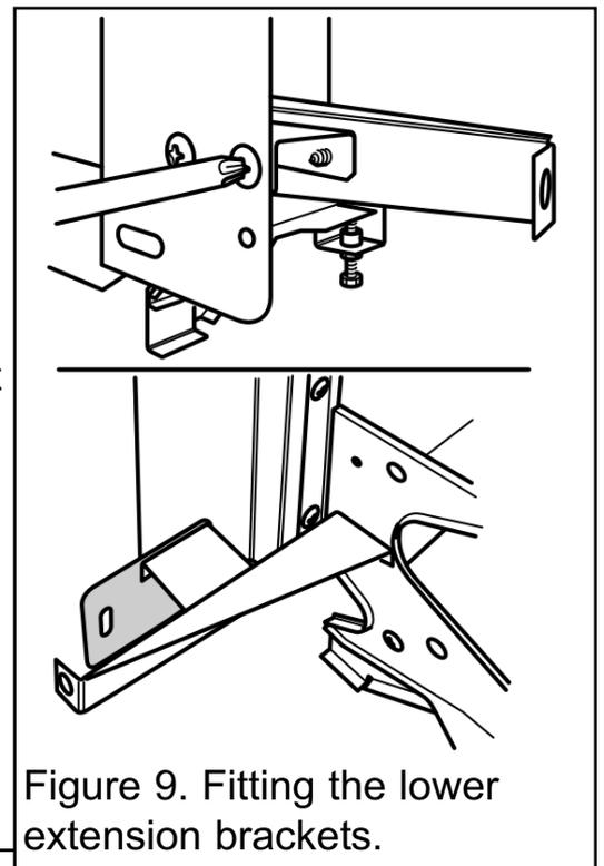
Figure 9. Fitting the lower extension brackets.
