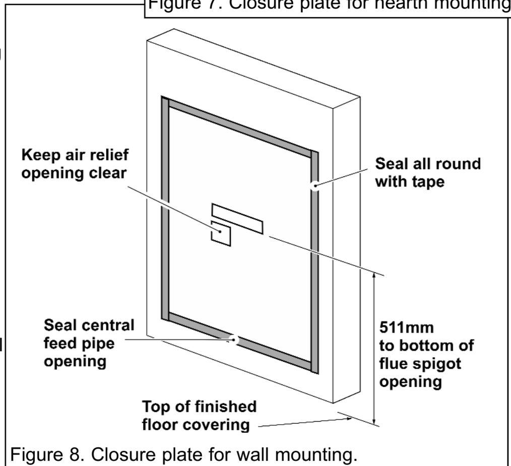
Figure 8. Closure plate for wall mounting.
