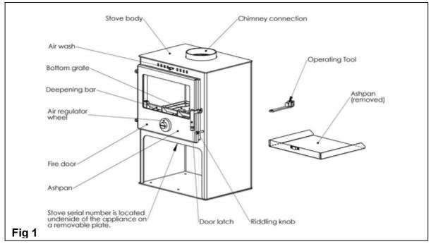
The highest burning rate is achieved by opening the air regulator wheel to maximum. Excess clinker formation may indicate overfiring.
