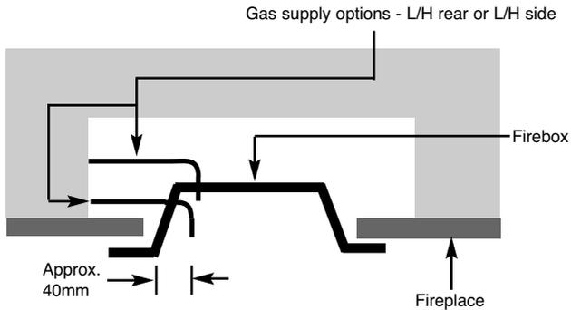
**Note : Before breaking into the gas supply a tightness test should be carried out to establish that the existing pipework is sound.**
