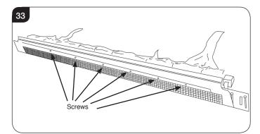
7.25 Remove the 10 self tapping screws that secure the Effects bar to the back of the appliance, see Diagram 34.
