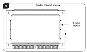
4.2 Loosen or remove the remaining brackets in order to slide off the outer decorative and effect screens. Using two hand remove the screens, see Diagrams 4 & 5.
