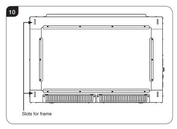
3.2 To remove the frame lift carefully and pull forward.
