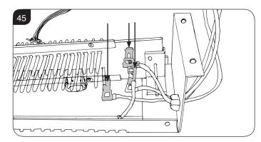
8.9 Remove the two screws on the underside of the element bracket (one at each end), see Diagram 46.
