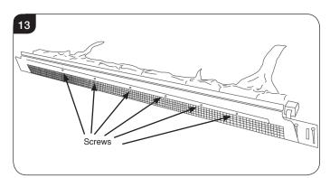
6.12 Remove the 10 self tapping screws that secure the Effects bar to the back of the appliance, see Diagram 14.
