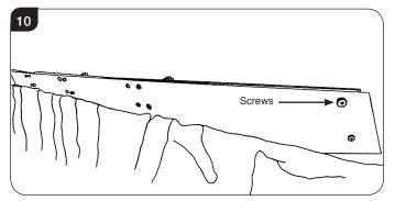
6.7 Remove the screws and washers and place carefully to one side for reuse later, see Diagram 11. NOTE: These parts are extremely small and delicate so care
