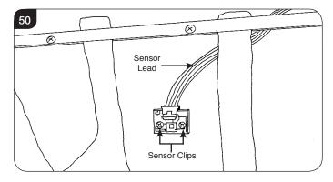
9.4 Remove the sensor and replace as required.
