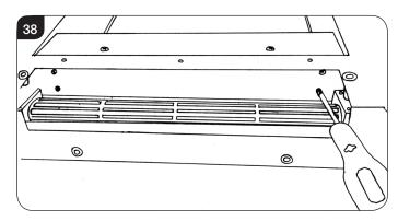
7.29 Remove the screws in the side panel and lift the fan unit out of the appliance, see Diagram 39.
