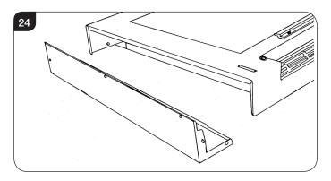
7.10 Stand the appliance upright and holding the right hand side turn the casing through 90 to reveal the appliance controls, see Diagram 25.
