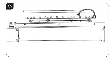
7.30 Remove the Upper & Lower LED boards from the fan and remove fan from the bracket by removing the screws in the top, see Diagram 40.
