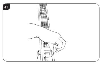
8.4 Remove the screws on the back which secure the flame effect bracket, see Diagram 42.
