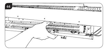
8.8 Carefully remove the wires on the right hand side using long nosed pliers making note of the wiring positions, see Diagram 45.
