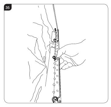
7.26 Using a pair of long nosed pliers remove the board from the plastic pegs securing it to the fan assembly, see Diagram 36.
