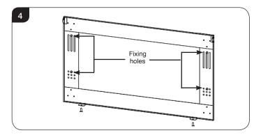
2.9 Drill the 4 holes and insert the rawlplugs provided. Note: The rawlplugs supplied are suitable for solid wall applications. If it is intended to mount the appliance onto plasterboard or hollow walls suitable fixings must be used, see Diagram 5.
