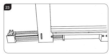
7.7 Replace fan units in the reverse order. DO NOT OVER TIGHTEN SCREWS.
