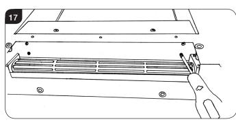
6.17 Note the orientation of the LED board and the connecting plugs. Using a pair of long nosed pliers remove the board from the plastic pegs securing it to the flame effect cloth, see Diagram 18.
