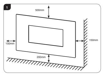
2.6 Decide on the height from the floor level to the bottom of the decorative frame (minimum of 200mm). Add the desired distance between the bottom of the frame and floor level to the frame dimension 'D' in Diagram 3 (see table over page) to achieve the total distance in Diagram 2. This will give the required height to the underside of the wall mounting bracket.
