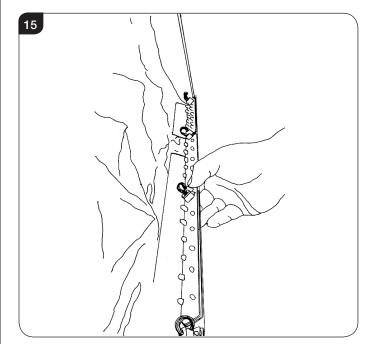
6.13 Using a pair of long nosed pliers remove the board from the plastic pegs securing it to the fan assembly, see Diagram 16.
