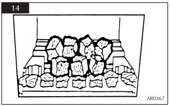
6.11 Place two small coals at each end of the front coal so that they lean against the flame baffle, and a further two large coals on the flame baffle, one at each end, see diagram 15.
