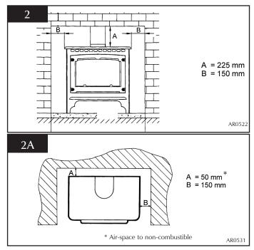
The above dimensions provide adequate clearance at the side and rear of the fire so that the controls can be reached.
