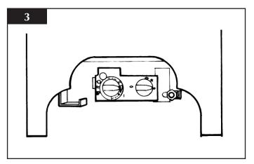
There is a cutout in the RH rear leg to enable a direct straight connection to be made to the rear of the stove. See diagram 3. A gas soundness check must be completed up to the gas inlet connection.
