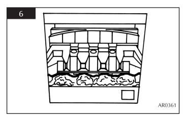
6.4 Place five of the loose round coals on the front coal so that they lean against the flame baffle, in between the fingers. Place the two rectangular coals behind the round coals, one at each side, see diagram 7.
