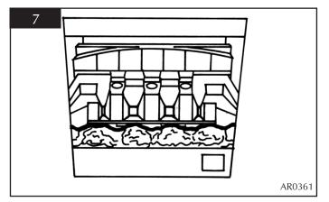
6.4 Place five of the loose round coals on the front coal so that they lean against the flame baffle, in between the fingers. Place the two rectangular coals behind the round coals, one at each side, see diagram 8.
