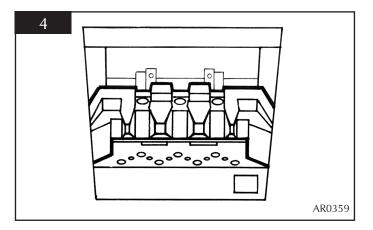
6.2 Locate the rear panel against the spacer brackets and slide down so that it locates on the ledge of the flame baffle, see diagram 5.
