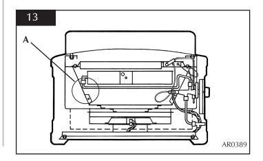
8.2 Rotate the injector until it is fully removed, and install the correct replacement injector. Reassemble and turn the gas supply on, check for leaks.
