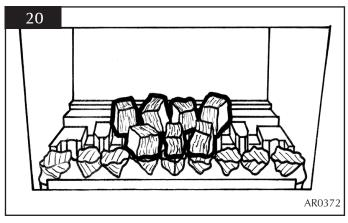
6.17 Place three small coals at each end of the front coal so that they lean against the flame baffle and a further four large coals on the flame baffle, two at each end, see diagram 21.
