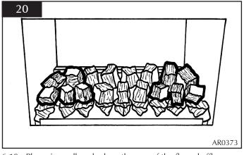
6.18 Place six small coals along the rear of the flame baffle, resting against the rear ledge, see diagram 21. NOTE: ENSURE THAT THE COALS ARE POSITIONED, AS DETAILED ABOVE. ONLY USE THE CORRECT AMOUNT OF COALS, AS SPECIFIED IN THE DIAGRAMS.
