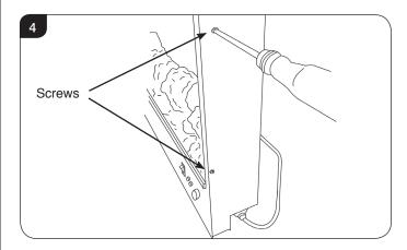
5.3 Remove the 4 screws on the back (2 on either side of the back), see Diagram 5.
