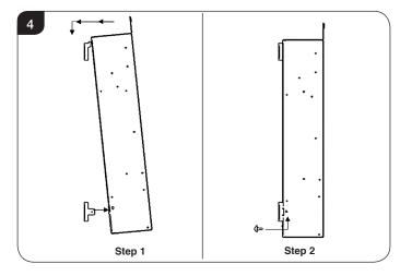
2.24 Use two No.6 x 12 screws from the kit to fix the fire through both sides into the holes in the lower bar.
