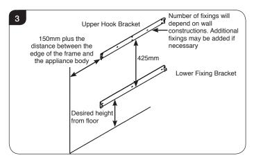
2.20 Use a spirit level to check the bars are straight. Mark the positions for the retaining screws. Remove the bracket and drill the holes
