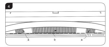
Dust build-up can inhibit efficient performance of the fan and lead to the safety cut-out operating.
