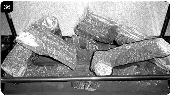
8.21 Once the logs are in place use some of the Embaglow wire wool provided and cover the ports in the burner tray with a liberal amount of fibres, in the highlighted areas shown in Diagram 37.
