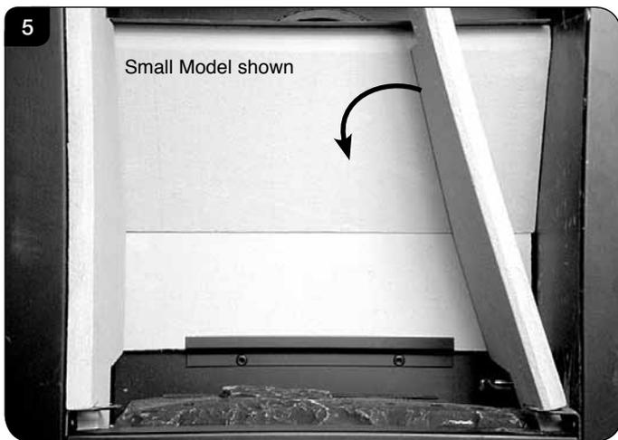
4.5 To remove the Right Hand liner first tilt inwards towards the centre of the firebox before lifting up and pulling out through the front of the firebox, see Diagram 5.
