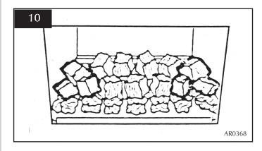
3.12 Place five small coals along the rear of the flame baffle, resting against the rear ledge, see Diagram 11.
