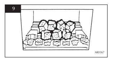
3.12 Place two small coals at each end of the front coal so that they lean against the flame baffle, and a further two large coals on the flame baffle, one at each end, see Diagram 10
