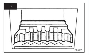
6.2 Locate the front coal moulding in front of the flame baffle ensuring that the end legs sit flat against the burner skin, see Diagram 4.
