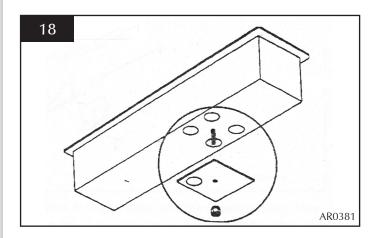
10.3 Remove the plate and replace with the correct size, ensure that the hole(s) in the plate align correctly with the holes in the underside of the airbox and replace the Nyloc nut.
