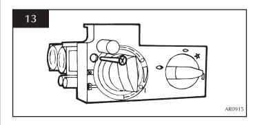
6.4 To release the right-hand side of the control cover, insert the narrow blade screwdriver into the slot shown in Diagram 11. Lever it gently and pull from the right-hand side at the same time. The cover will now come off. There is a small cylindrical metal spacer inside the cover. This must be kept and replaced on the fixing screw during re-assembly.
