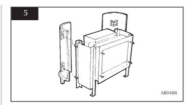
3.8 Remove the cast iron door using the tool provided, and carefully place to one side. Gently position the front ceramic panel so that the side panels locate inside the returns on the front panel, engage the bolt heads in the brackets on the back of the panel and gently slide into place so that the ceramic comes to rest on the floor, ensure that the opening in the panel sits centrally around the fire box opening, see Diagram 6.
