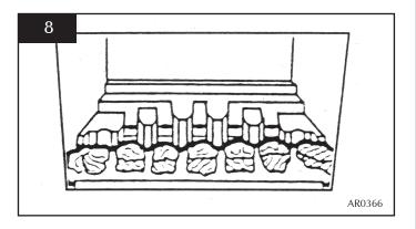
3.11 Place three large coals on the front coal so that they lean against the flame baffle, and the four large coals on the flame baffle so that they sit on the fingers, see Diagram 9.
