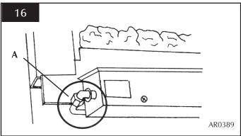
8.2 Rotate the injector until it is fully removed, and install the correct replacement injector. Reassemble and turn the gas supply on, check for leaks.
