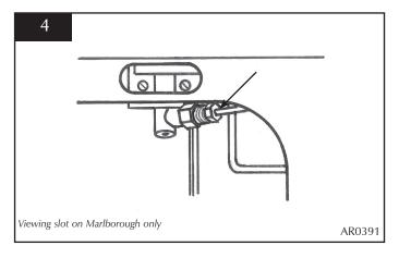
2.2 Disconnect thermocouple from gas valve. See Diagram 2. Remove ignition lead from electrode. (Cut cable tie to ignition lead if required).
