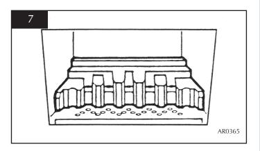
3.10 Locate the front coal moulding in front of the flame baffle ensuring that the end legs sit flat against the burner skin, see Diagram 8.
